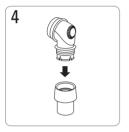
Remove the swivel from the elbow.
