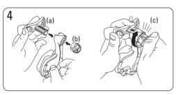
Insert the forehead support (a) into the mask frame and screw (b) the dial clockwise onto the pole. Turn the dial until it clicks (c). Ensure the dial sits flush against the frame.
